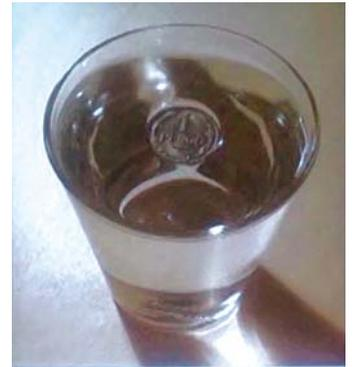
Fig. 16.1 Evidence of water's high surface tension
